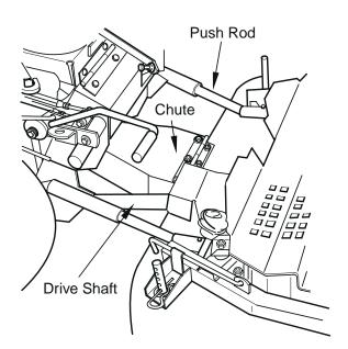
Figure 4-18 Aligning Deck With Push Arms
